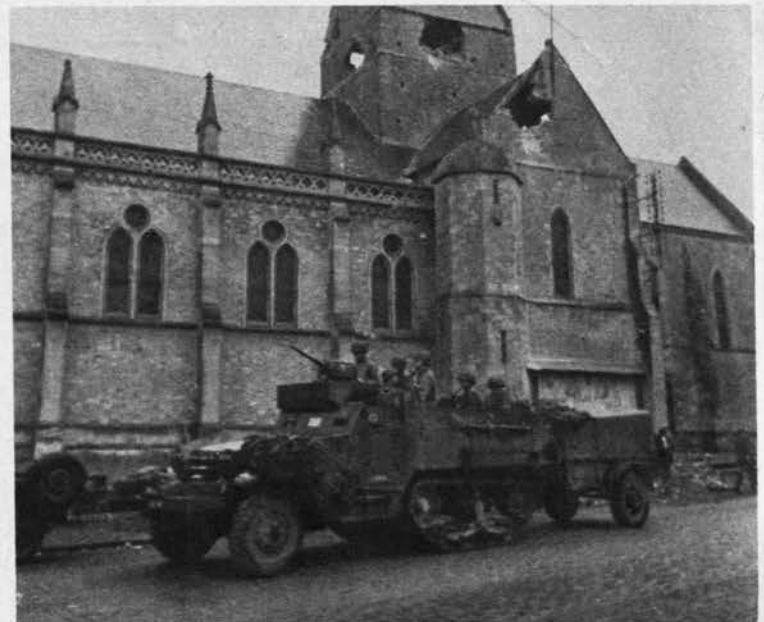
Transporting personnel is one of the M-3 half-track's main functions. It can carry a rifle, mortar or machine-gun squad. The ring-mounted MG above the cab identifies this version as the M-3A1 half-track.
